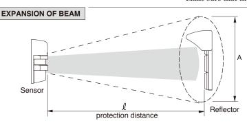
Expansion of beam can be calculated as follows. A=0.03  $\times$  [/
