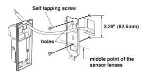
Pull the wire through the sensor body (back to front) and attach it to the terminals on the sensor.
