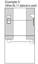
\*The sensor and reflector units should be installed uprightly and vertically.
