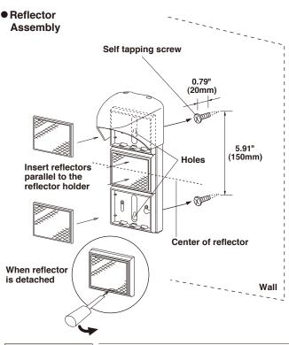
①Insert self tapping screws into the wall by about 0.79" (20mm) and hang the reflector unit back plate on them using the holes.
